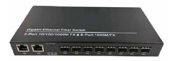
The compact and sleek metallic enclosure also acts as a heatsink, making this device passively cooled - no fan noise and no dust accumulation inside. Special rackmount ears for installing unit into the standard rack are provided.
